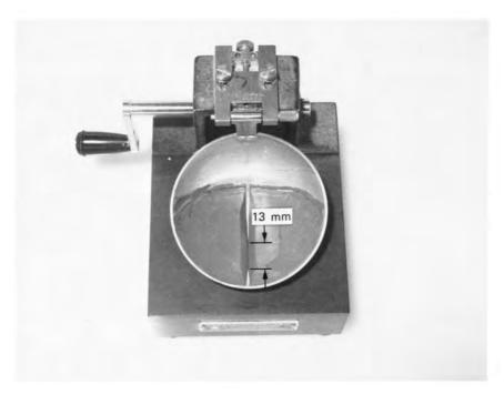
FIG. 8 Soil Pat After Groove Has Closed
